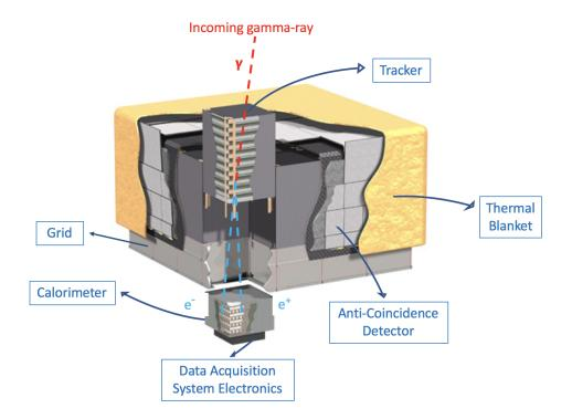
Figure 3.3: Schematic illustration of the Fermi-LAT instrument. Figure adopted from [155]
